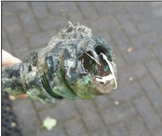
Leak - Poor Quality Joint
